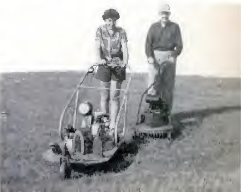
Two 20-inch mowers go to work on the lawn. The one at the left is converted from the miniature auto
